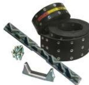
The X track cleat combines a steel core with a high quality vulcanized rubber encasement. The rubber encasement has a herring bone structure that provides the cleat with excellent grip. The rubber is abrasive resistant against dirt and rocks that become exposed on the trail system.
