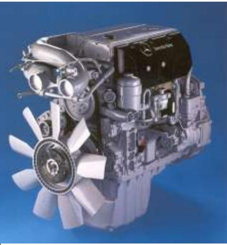
With its new OM 924 LA 4.8 liter diesel engine from Mercedes-Benz with turbocharger and charge-air intercooler the TrailBully now has even more power. State of the art high pressure fuel system, advanced electronic engine management and three valve technology yields an output of just under 200 horsepower. The OM 924 LA is rated Tier 3 for low exhaust emissions and is thrifty on fuel. The drive line features a Rexroth hydrostatic transmission for high thrust, high maximum speed and durability.
